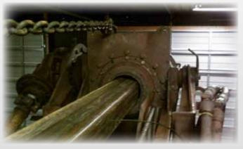
Texoma 700 drilling rig main gearbox
