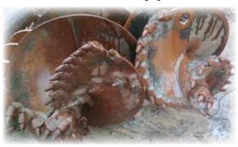
Rock drill auger bits for drilling tough rock strata. Using bits like this, Ransom can drill holes from 12 to 36 inches in diameter.
